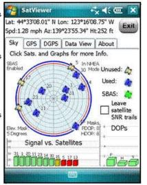
configuration and settings. The screen to the right shows the SatViewer's Sky Plot, a graphical representation of where available satellites are in the sky, and what their signals strength is. SatViewer is not itself a mapping or GIS application, but it definitely helps to get the best performance out of the GPS receiver.
